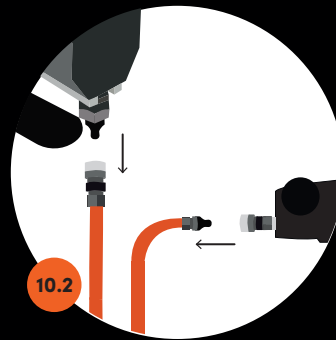
Disconnect the hydraulic hose from the Lokring tool and the Hydraulic pump
